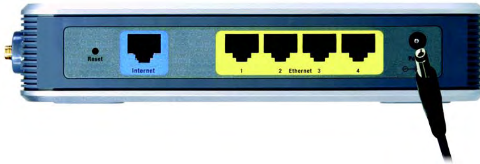
Figure 4-3: Connecting the Power
